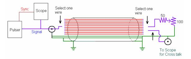
The Kerpen cable is not a coax cable and hence does not provide constant impedance. The impedance of a particular wire depends its location with respect to the ground shield and the ground wires in the cable bundle. We picked a random combination and checked some ten wires to obtain the following results:
