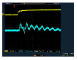
Same configuration but wire #6 and #16 are now connected at the far end (which would be the case if the two wires share the same HV channel).
