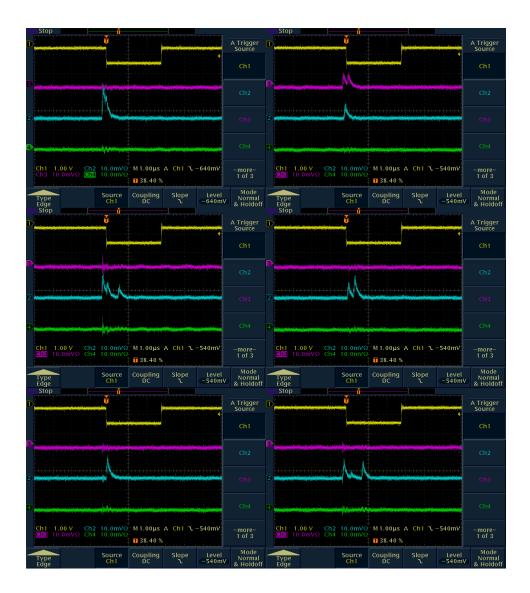
Same configuration as before but this time without the 82 Ohm termination resistor. Ten typical pulses (the vertical scale is 10 mV for the green, blue and purple traces)
