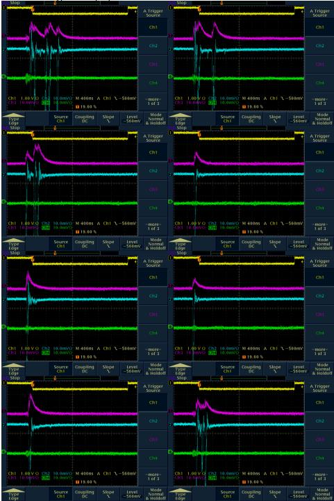
We further studied the performance of the base line solution by recording the pulses (green trace) from a far away strip and not from a neighboring channel (same tube, other side). Here are 10 typical scope pictures.
