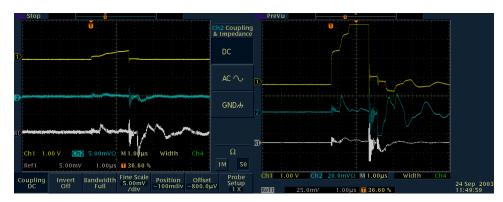
The observed cross talk is very small. It can be further reduced by terminating the HV cable at the power supply end with 80 – 100 Ohm which matches the average impedance.
