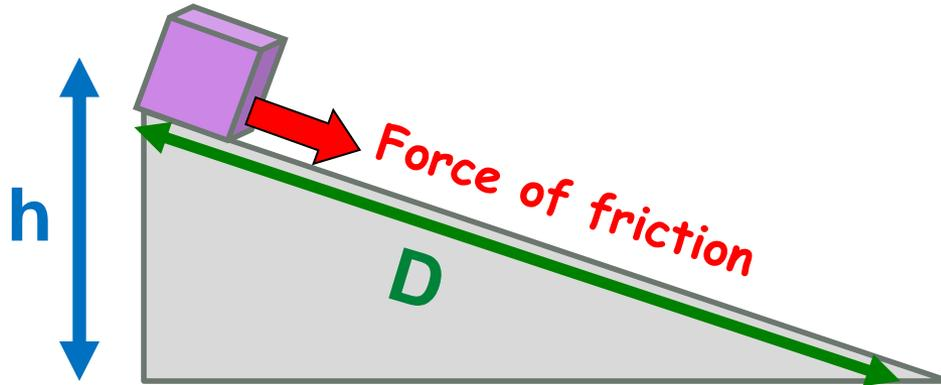
$$W = F \text{ (friction)} \times D \text{ (length of ramp)}$$
